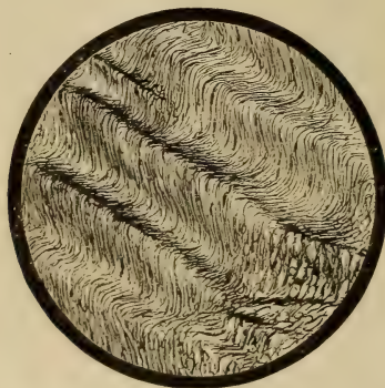
FIG. 19.—CONTORTED MICACEOUS-SCHIST, AS SEEN UNDER THE MICROSCOPE WITH A MAGNIFYING POWER OF 50 DIAMETERS.
